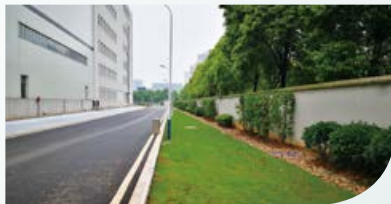
● Contiguous open green spaces naturally absorb and filter rainwater, avoid adjacent pavements from overflow in heavy downpours
